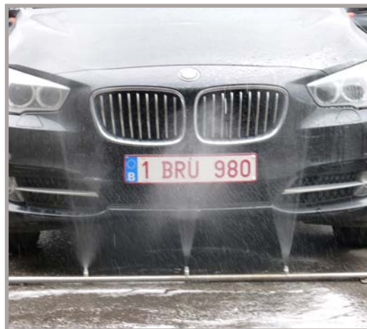
Machine HP désallage
